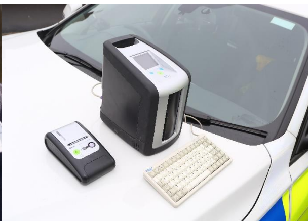
Drager DDT 5000 with printer and keyboard.
